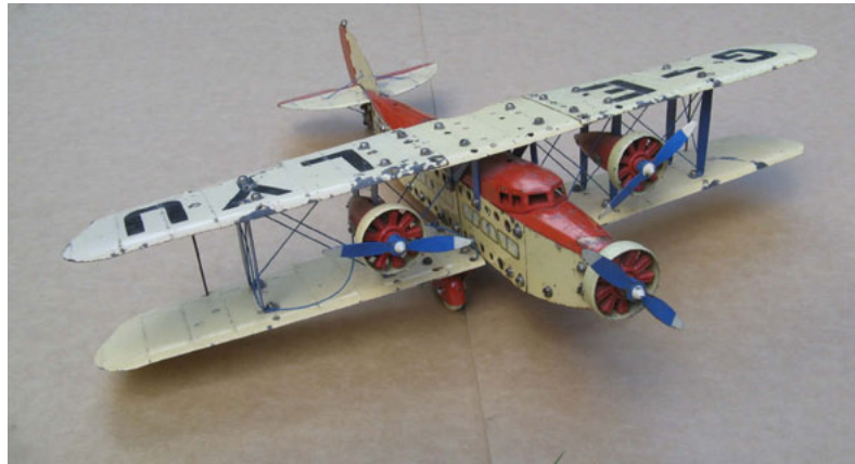
A three-engine biplane airliner made from the Special Aeroplane Constructor Outfit No 2. Extras in this Outfit include a cabin for the pilots, and "Townend rings", cowlings around the radial engines. These rings were invented by Dr Hubert Townend and patented in England in 1929. They reduced the drag of radial engines and also added some forward thrust
