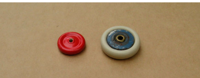
Two of the special Aero Outfit wheels. The blue wheel has a boss in between its two faces. To get to the grub screw, you need to peel back the tyre and insert the Aero set screwdriver, which is not flared near the blade (this screwdriver can also be poked through Meccano holes)
